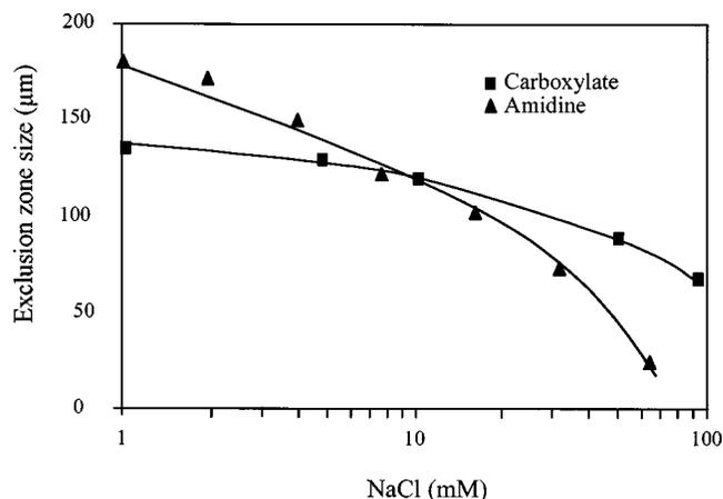
FIG. 7. Effect of salt on the exclusion-zone size with 2- $\mu\text{m}$  carboxylate and 1.5- $\mu\text{m}$  amidine microspheres suspended in aqueous solutions at  $p\text{H}$  2.5 and  $p\text{H}$  10, respectively.
