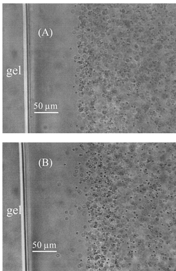
FIG. 5. Comparison of results obtained with microspheres of opposite charge. (A) 2- $\mu\text{m}$  carboxylate microspheres, negatively charged. (B) 1.5- $\mu\text{m}$  aldehyde/amidine-coated surface, positively charged.
