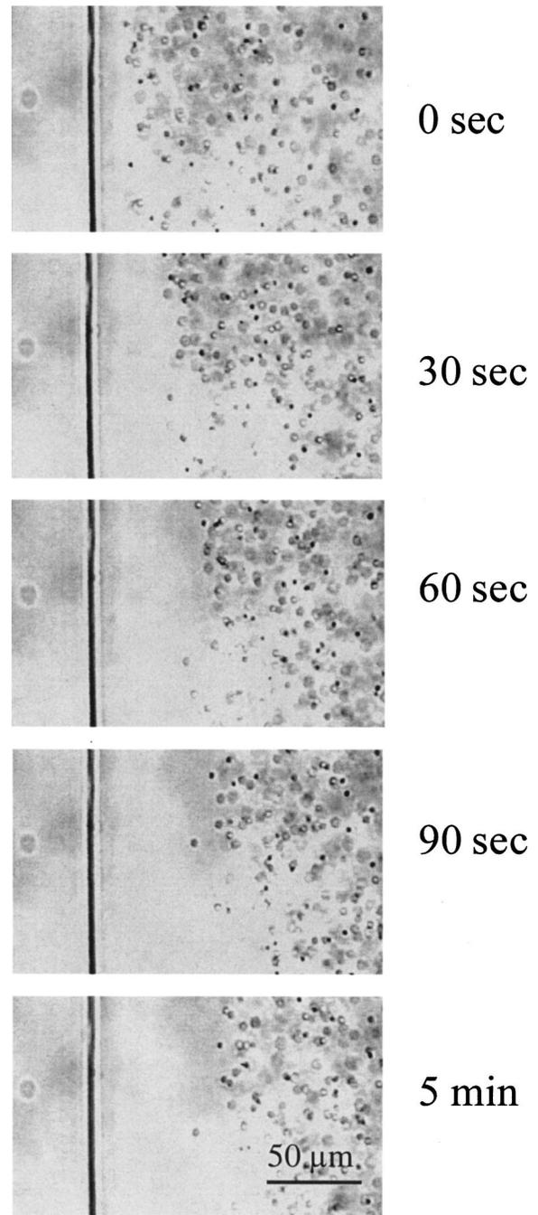
FIG. 3. Development of an exclusion zone as a function of time in a cylindrical channel of a PVA gel. Carboxylate-coated microspheres,  $2\ \mu\text{m}$  in diameter, were used.
