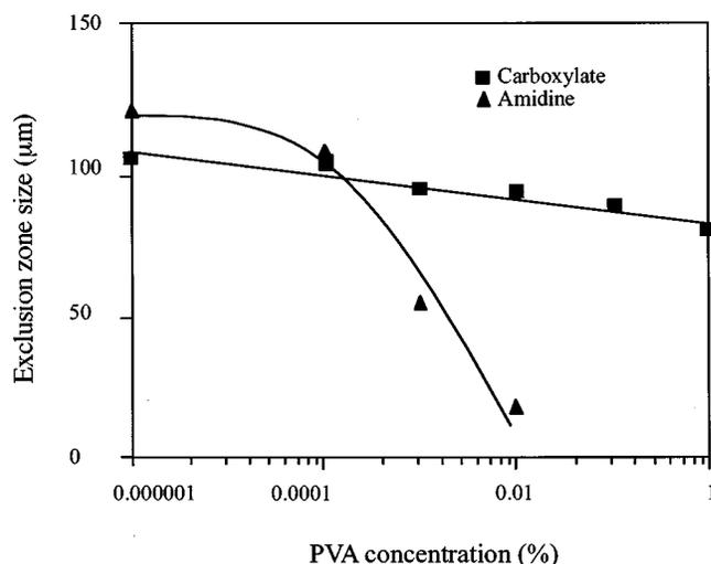
FIG. 4. Effect of PVA molecule concentration on exclusion-zone size using  $2\text{-}\mu\text{m}$  carboxylate and  $1.5\text{-}\mu\text{m}$  amidine microspheres, which were suspended in PVA solutions at  $\text{pH } 10$  and  $\text{pH } 2.5$ , respectively. Curves are drawn as a guide.
