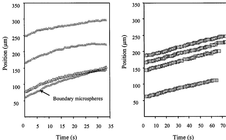
FIG. 11. Time course of exclusion of 1.5- $\mu\text{m}$  amidine microspheres in solution at  $p\text{H}$  2.5 (left) and 2- $\mu\text{m}$  carboxylate microspheres in solution at  $p\text{H}$  11 (right), after exposure to the PVA gel surface. Different traces show the behavior of microspheres at different initial separations from gel.
