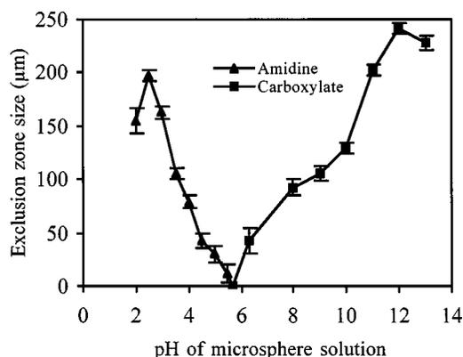
FIG. 6. Effect of  $p\text{H}$  on the size of the exclusion zone, where 2- $\mu\text{m}$  carboxylate microspheres and 1.5- $\mu\text{m}$  amidine microspheres were suspended in aqueous solution at different  $p\text{H}$ . PVA gels were stored in pure water at  $p\text{H}$  5.7. Note: microspheres of slightly different size were used because the same sizes were not available in amidine and carboxylate. Curves are drawn to guide the eye.
